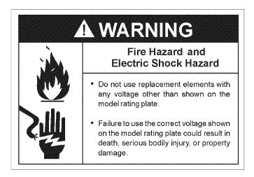
Replacement elements must (1) be the same voltage and (2) no greater wattage than listed on the model rating plate affixed to the water heater.
